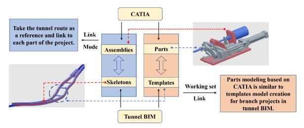
Fig. 2 - Comparison of CATIA and tunnel BIM
