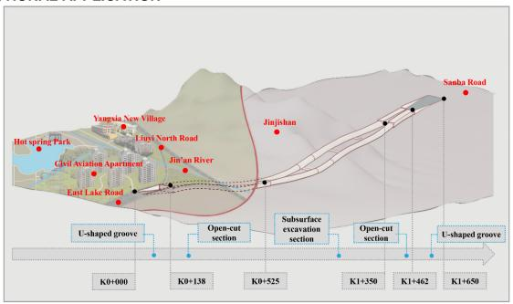
Fig. 10 - CATIA-based BIM model of Jinjishan tunnel
