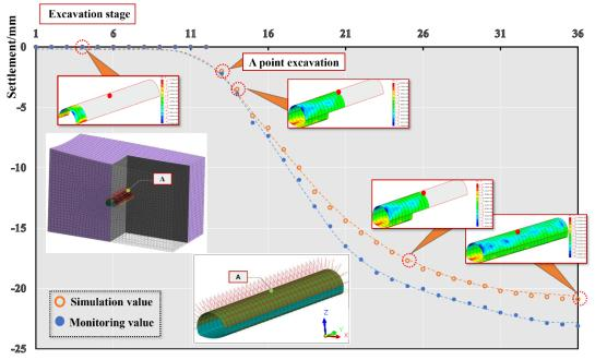
Fig. 13 - Comparison of simulation value and monitoring value
