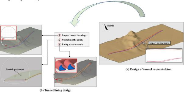
Fig. 6 - Tunnel skeleton design
