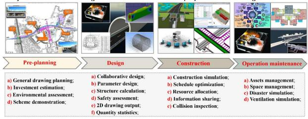
Fig. 1 - The role of BIM in different stages of the project
