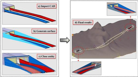
Fig. 8 - Modeling process of U-shaped groove
