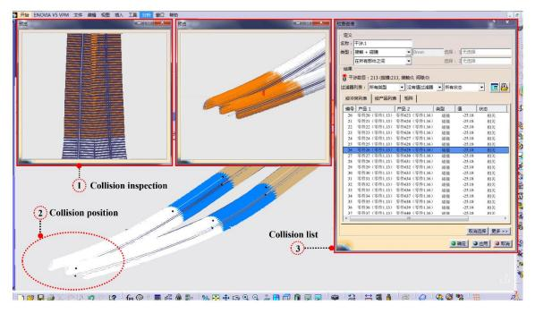
Fig. 11 - CATIA-based tunnel bolts collision inspection
