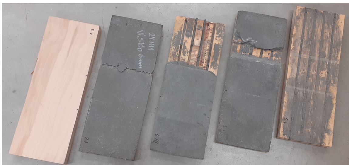
FIGURE 3. View on the damaged representative specimens after the loading test, one from each group D.1 to D.5. For group D.3 and D.4, the HPC was removed after the testing to see the ribs and the positive influence of the transverse rib.
